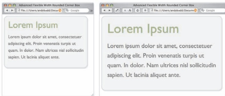
Figure 4-9. Flexible rounded-corner boxes expand both horizontally and vertically as the text is resized.
